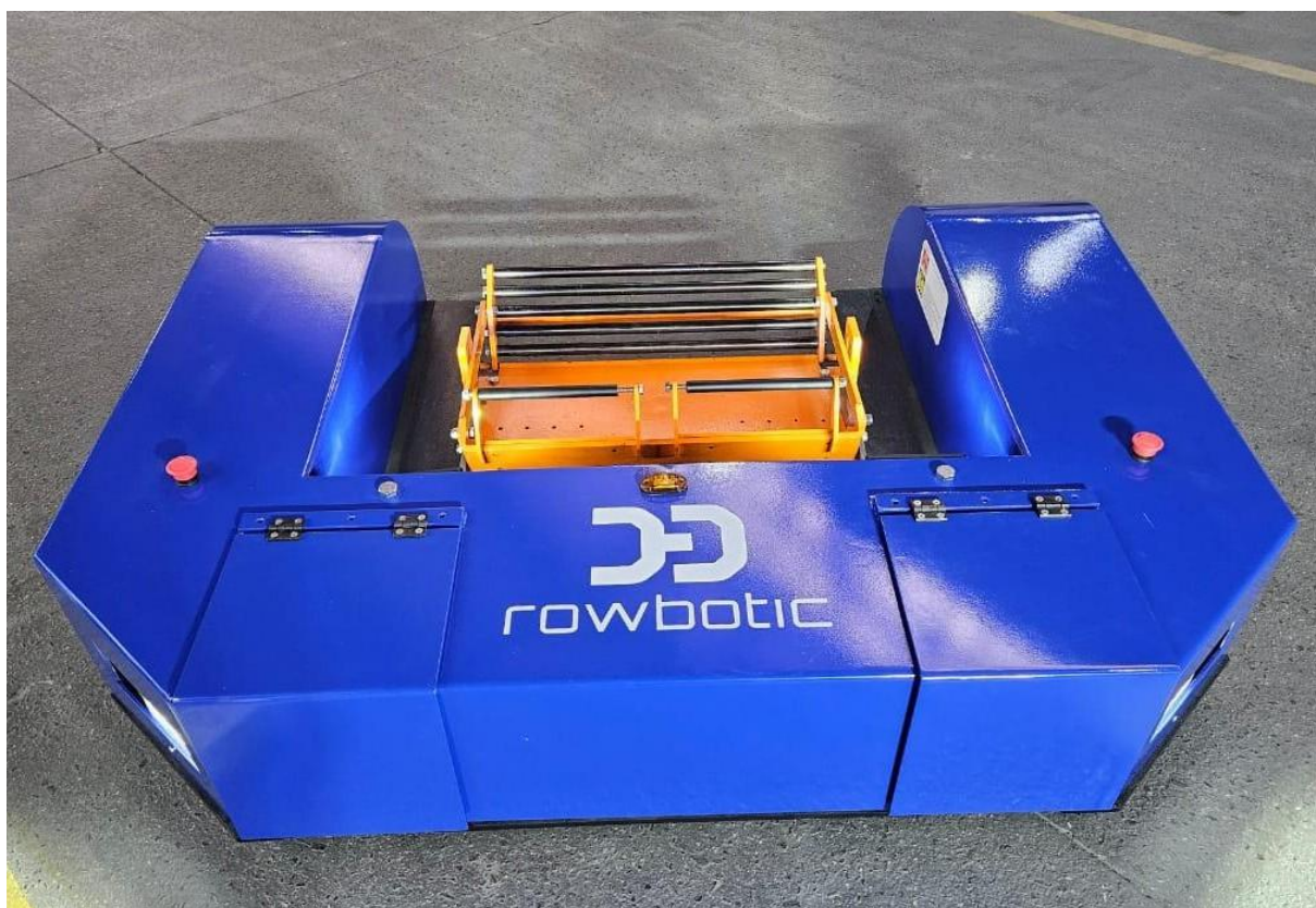
Figura 3: Vista superior do TowPower TP50 mostrando as tampas dos compartimentos e a marca Rowbotic
